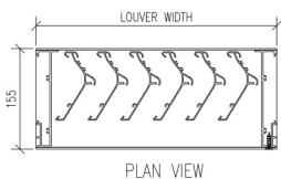
TWY420F  $\frac{\text{Discharge Coefficient}}{\text{Cd} = 0.26 \text{ (Class 3)}}$
